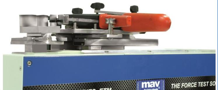
The KBP-A tool enables a continuous testing due to the electromotive drive of the machine's load sled. The options force preset, movement path preset and testing speed preset can be chosen and adjusted.
