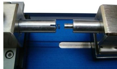
*Circuit Board Pressure Testing Tool*
