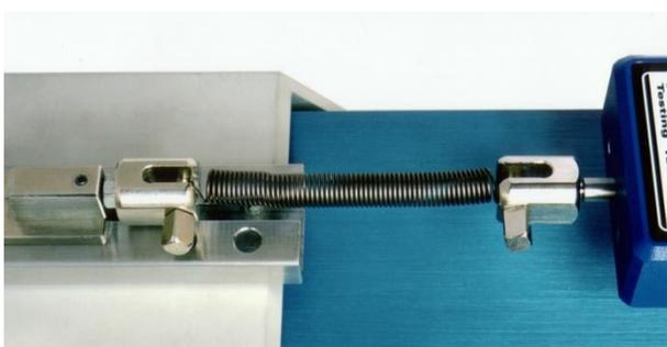
*Testing Tool for Compression Springs*
