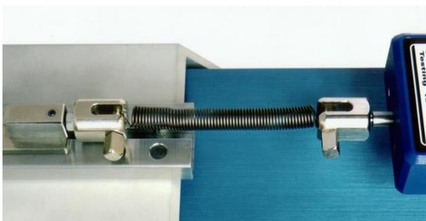
*Testing Tool for Compression Springs*
